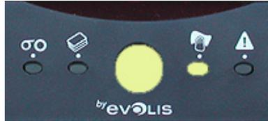
Although it is recommended you clean the printer with every ribbon change, the Badgy has an alert message to warn you that cleaning is required. The cleaning light on the control panel will illuminate (after 400 cards).
